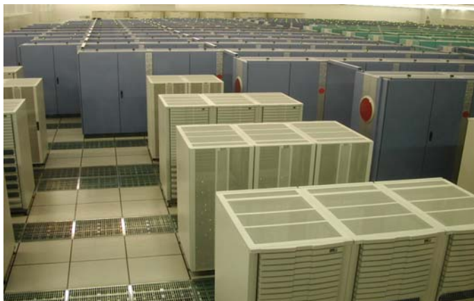
The earth Simulator. Each blue box is a node containing 8 CPU's
