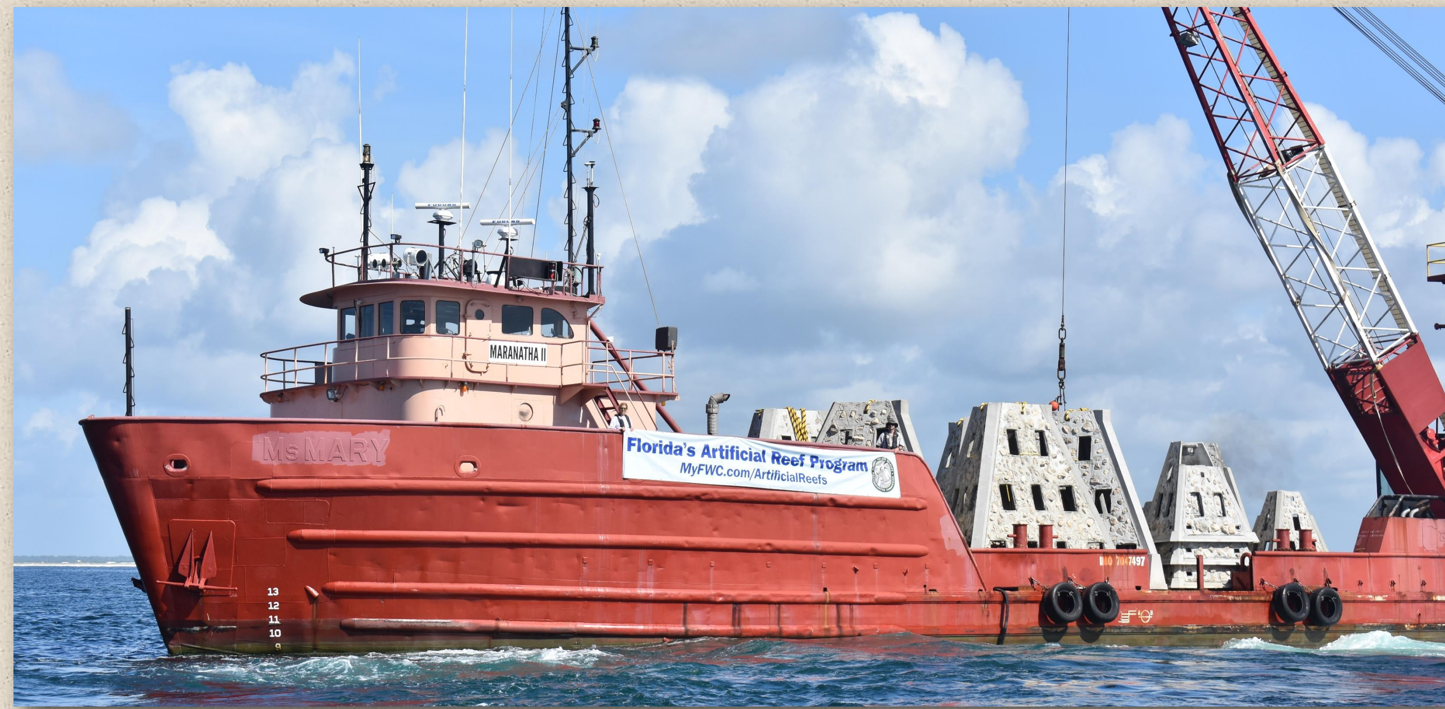
Figure 1. Deploying 8 and 15 ft. tall modules. Hydrophones are attached to these types of modules post-deployment.
