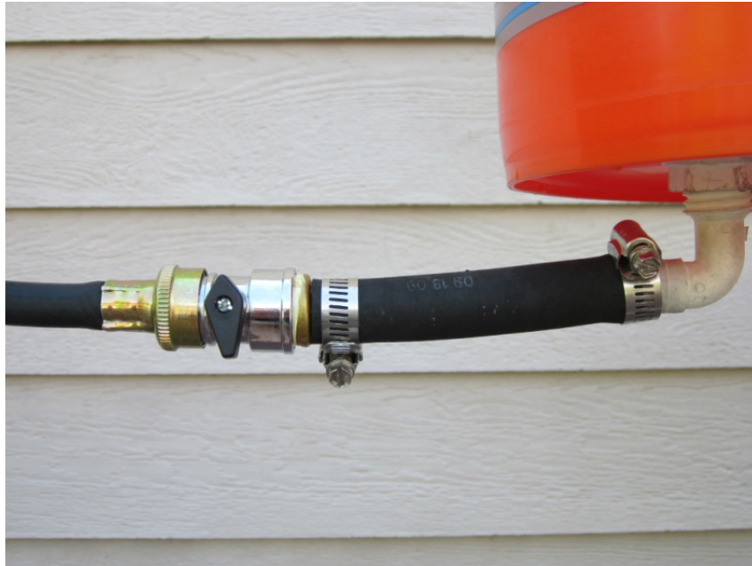
APPENDIX FIGURE 3. Drip bucket reservoir showing hull fitting, ½-inch hose with clamps, cut-off valve, and garden hose attachment.
