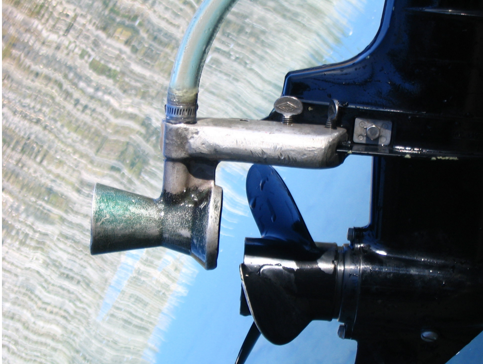
FIGURE SOP 11.5. Close-up view of venturi attached to cavitation plate and tightened down using wing screws for quick installation/removal.
