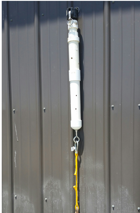
FIGURE SOP 5.2. Example of a weighted diffusion nozzle for deep-water applications.
