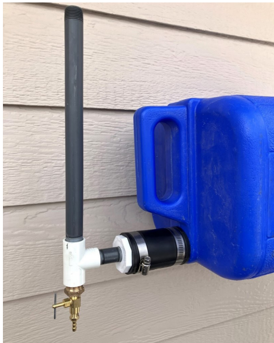
APPENDIX FIGURE 6. Completed drip can tipped on its side and ready for operation.
