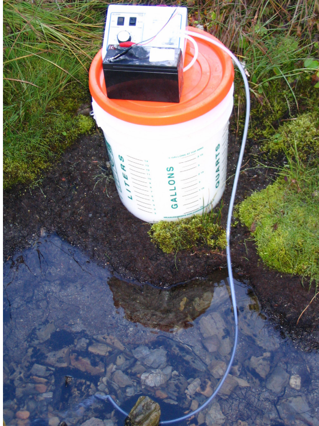
FIGURE SOP 11.3. Control Company peristaltic pump placed on rotenone bucket showing dispensing tube into stream. A 9-V battery sits alongside the pump.
