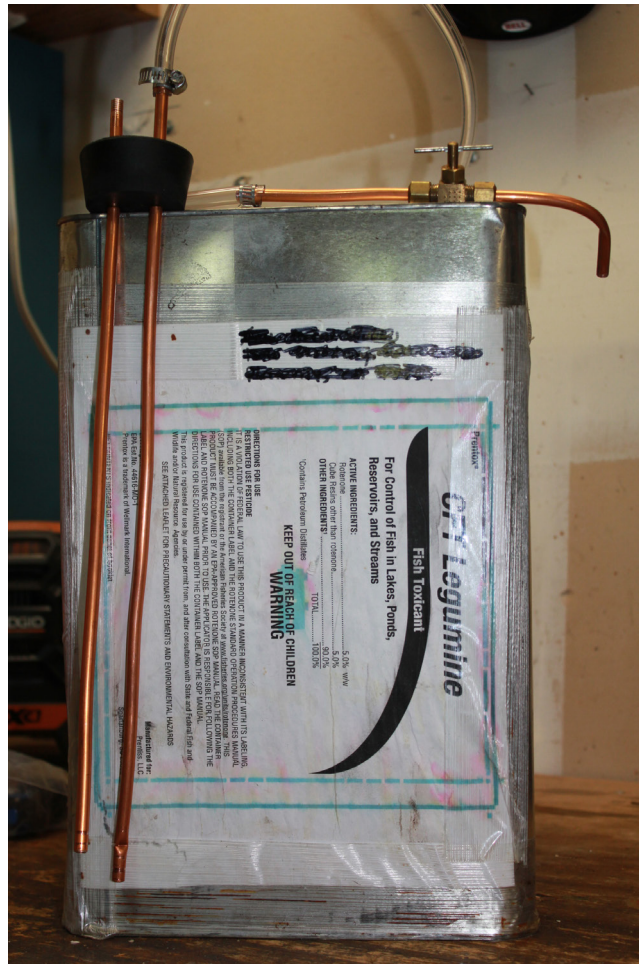
APPENDIX FIGURE 1. Drip can as service container showing placement of copper tubes (Pieces A and B) in rubber stopper and needle valve assembly attached to longer copper tube (Piece A) by Tygon tubing.
