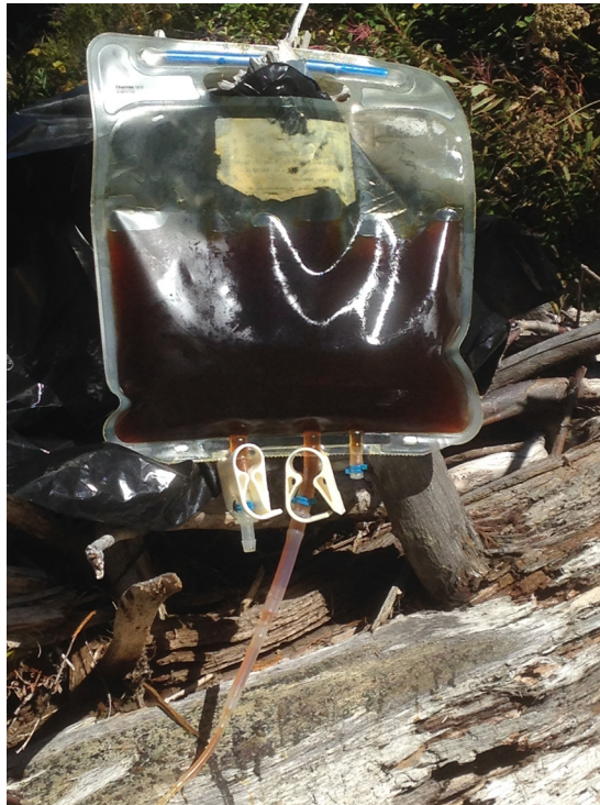
APPENDIX FIGURE 8. Drip bag in operation, with black plastic covering removed for display. Notice lack of air in bag and ports which are clamped off.
