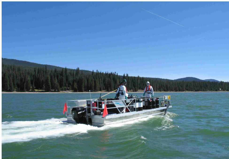
FIGURE SOP 8.4. Application of liquid rotenone below waterline using semi-closed application system at Diamond Lake, Oregon (Photo credit: Brian Finlayson, California Department of Fish and Game).
