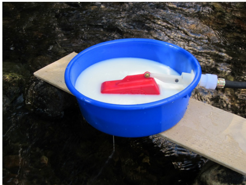
APPENDIX FIGURE 4. Dog watering bowl reservoir and float in operation. Feeder garden hose from drip bucket reservoir can be seen on right side of photo.
