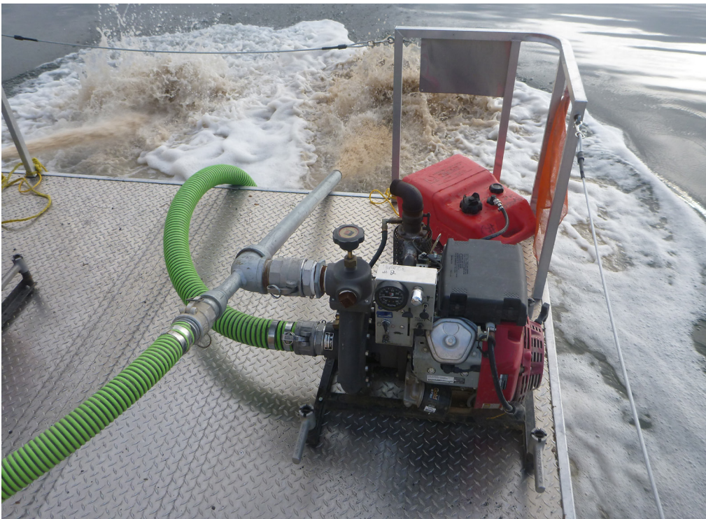
FIGURE SOP 9.3. Gasoline-powered water pump showing arrangement of intake and discharge hoses (Photo credit: Chad Jackson, Washington Department of Fish and Wildlife).
